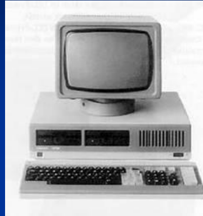
1986: PC 1715 8-Bit-Rechner, 64 K RAM Disketten, Graphikbildschirm, Wordstar, dBase, Pascal
