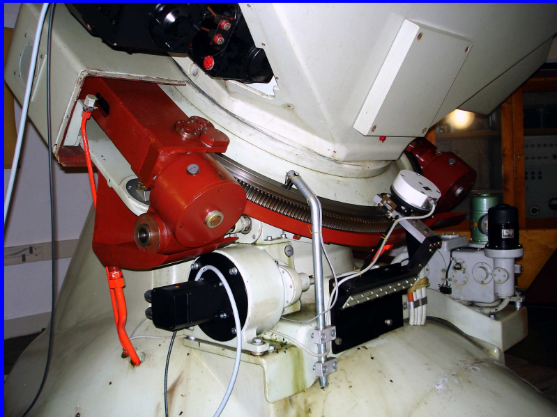
RA-Axis without protection cover with its servomotors and the Hall-Referencesensor
