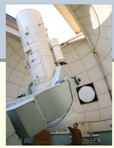
Xinglong National Astronomical O. 0.9/0.6-m telescope
