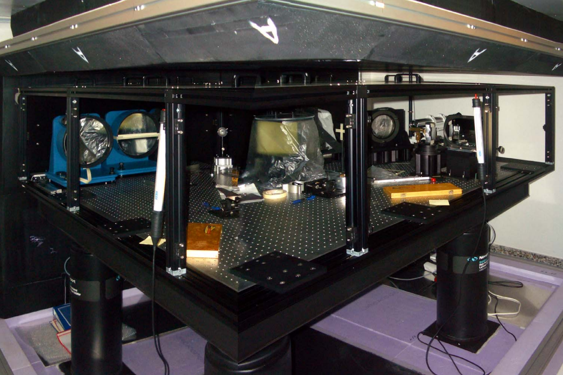
SES first-light version: R=55,000 , 390-870nm, E2V 2kx2k CCD.
