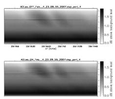
The sample of dynamic radio spectra (ON regime-lower panel, OFF regime-upper panel) of AD Leo obtained during the campaign at the UTR-2 with DSP. The zeropoint in the colorbar scale corresponds to the background level. The range is given in dB. This example shows the dynamic spectra and drifting structures (from higher to lower frequencies) but appearing too strong to be of stellar nature.
