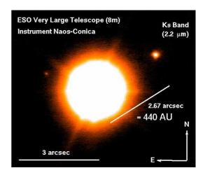
Deep, high S/N, high angular resolution VLT/NaCo image of CT Cha A (bright star in the center) and b (2.7 arcsec northwest of it) after shift+add of 30 observations of 28 sec each (March 2007). The object b is a planetary mass companion with a mass of few to 16 Jupiter masses. Northeast of CT Cha A a faint object can be seen, which is not co-moving, hence a background star.
